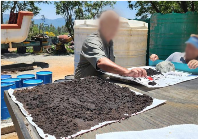
FIGURE 2 Samples being taken of Ilmenite concentrate and magnetite concentrates
